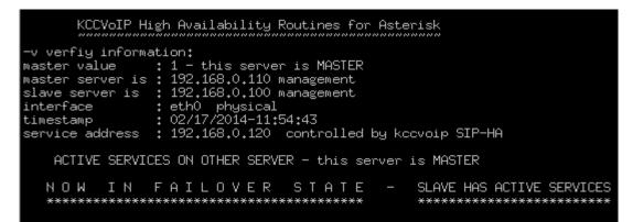
Then the operator issues the manual command on the slave server to force the service back in to the 'normal state' from the slave server (sip-ha -f) and replication will then continue in the master to slave direction
