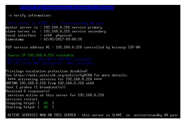
Notice the above example shows that the slave server will try to update the master server with all changes that are made to the active slave server during this failover condition so that both servers are kept in full synchronization and the master server will be up to date and ready to take over services again once normal state has been confirmed
